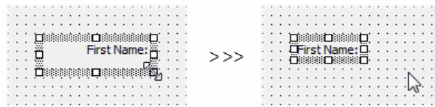
Fig. 7 Double-click the lower-right corner handle to snap the label to size.
